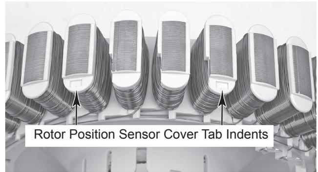
**REASSEMBLY NOTE:** When you reinstall the drive motor rotor over the stator assembly, do not grip the rotor housing around the rear edge with your fingers. The magnets around the rotor housing are very strong, and they will pull the rotor into the stator coil magnets when the rotor magnets come within their magnetic field. Keep your fingers along the outside of the rotor housing and away from the rear edge when you are installing it on the stator assembly.
