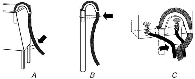
If the washer faucets and the drain standpipe are recessed, put the formed end of the drain hose into the standpipe. Tightly wrap the tie strap around the water inlet hoses and the drain hose. See view C.
