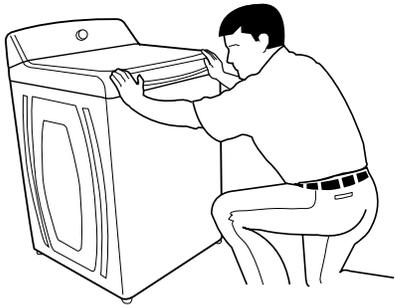
3. Lower right front foot until it contacts the floor. By hand, firmly rotate foot as much as an additional 1-1/2 turns. The other three feet have been preset at the factory.
