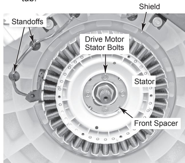
10. Disconnect the power connector from the stator terminals.
