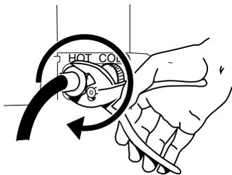
5. Attach the cold water hose to the inlet valve labeled cold.
