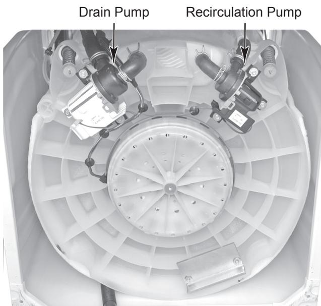
6. To remove the drain pump:
