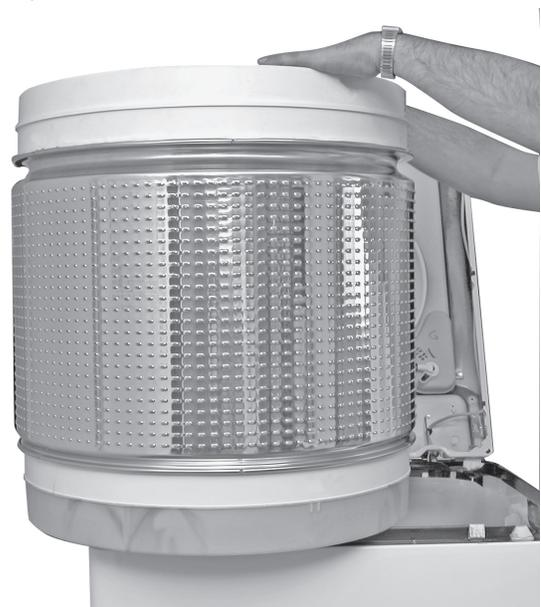
4. To remove the **basket hub**, remove the six screws, and lift the hub assembly from the basket.
