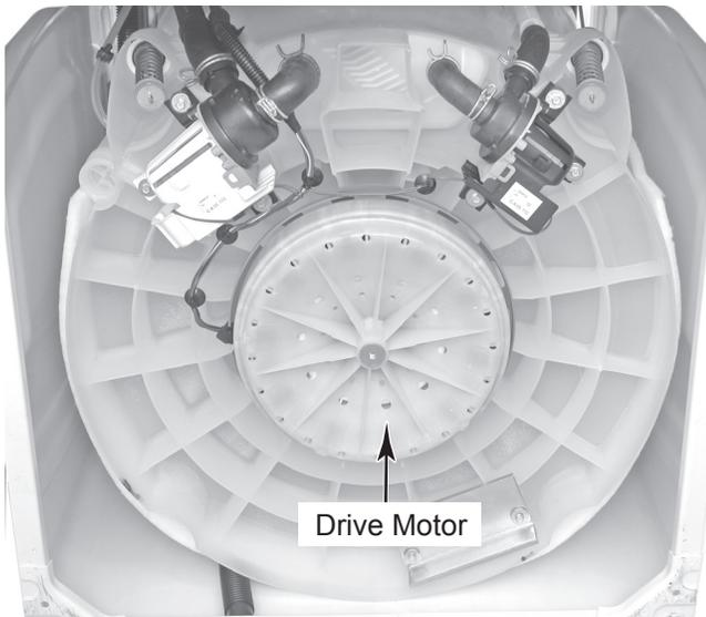
6. Use a 1/4" Allen wrench and loosen the rotor mounting screw as far as it will go (the screw is captive and cannot be removed from the rotor). The rotor is seated on the splined tub shaft. Rock the rotor back and forth and pull it off the shaft so it contacts the screw washer-head, then further loosen the screw. Do this until the rotor is removed from the shaft.
