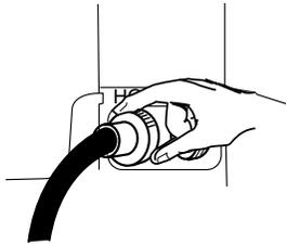
4. Using pliers, tighten the coupling with an additional two-thirds turn.
