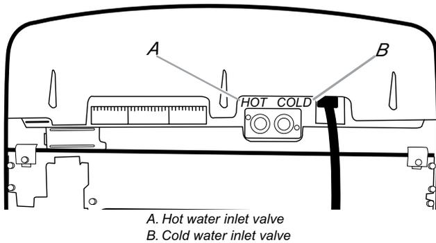
1. Attach the hot water hose to the inlet valve labeled hot.
