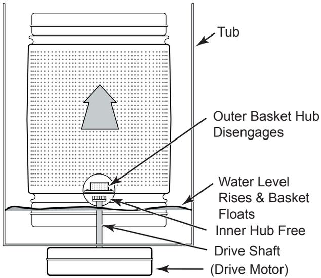
When the tub drains, the basket drops back to its original position, and the hub components re-engage, connecting the basket to the shaft, and permitting the basket to spin.
